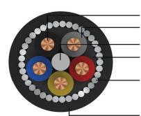
Soild Copper Conductor XLPE Insulation Filler (Optional) Inner Sheath
